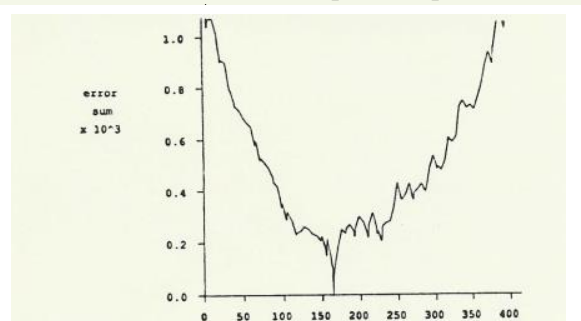
Fig (i) The merit function for a fine X-search scan along the "right" row. Note 16 pixel "dip" width.
