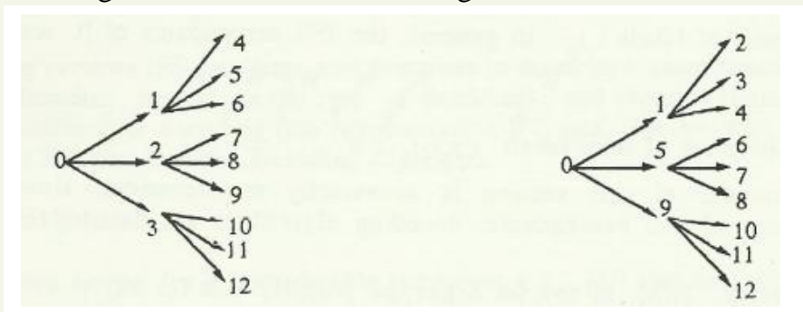
Fig 1 Sequence of marking of 2 generations of descendants from seed pixel 0 with 3 maps In the IFS set. On the left, generation-by-generation marking as for the Scanning Algorithms On the right, branch-by-branch marking as for the Stack Algorithm.
