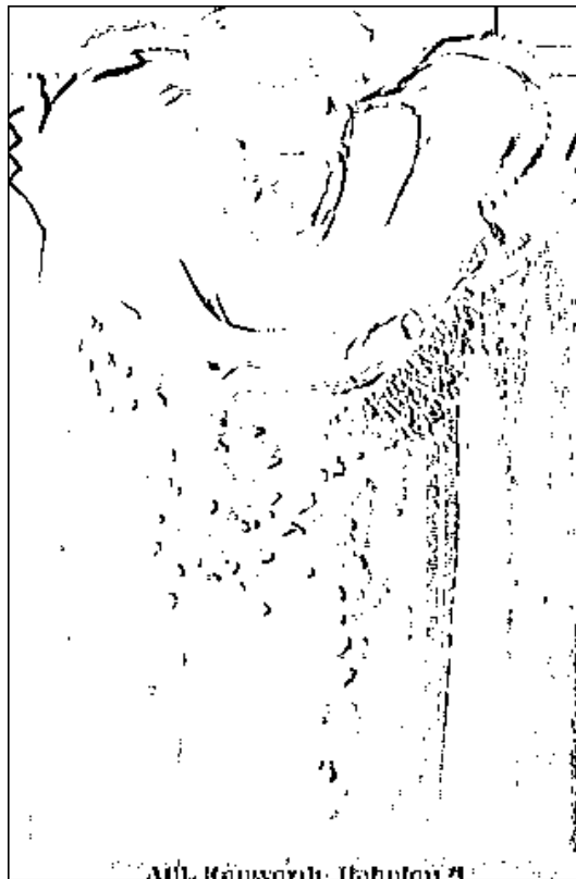
Figure 2: 316x500x24-bit colour Kosh: Output of Sobel edge detector applied on luminance (threshold T = 0.11). The original image has well defined edges involving small changes in grayscale. (See Fig 3)
