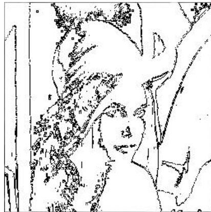
Figure 5: 256x256x8-bit Lena: Output of NN edge detector trained to duplicate "fuzzy" Sobel edgedness on 256 binary proto-types. Number of edge pixels = 7770.
